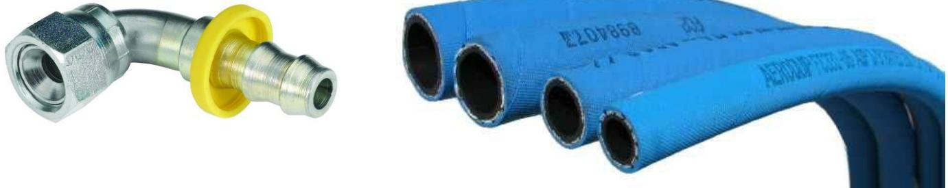
Howe Performance recommends using Eaton Aeroquip Low Pressure Push Lock style hose for all return lines. This is because the low pressure hose has a larger I.D. than high pressure hose and is less restrictive on the return line. It is similar to taking your thumb off the garden hose and letting the water free flow out. We use this in -8,-10 and -12 sizes.
